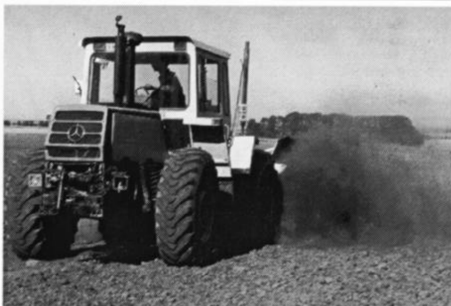
The rotary drainer in full swing. The laser guidance system allows the operator to follow the lowest point in the landscape.
